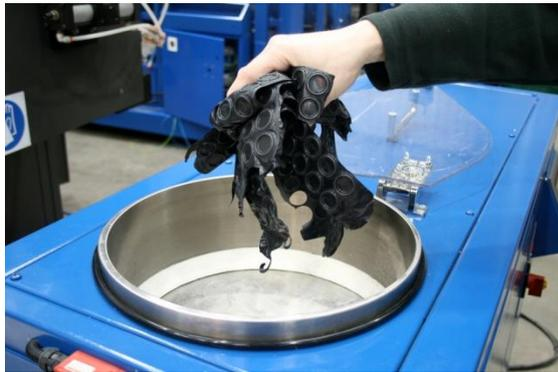
*Parts to be deflashed are dropped into the chamber*
