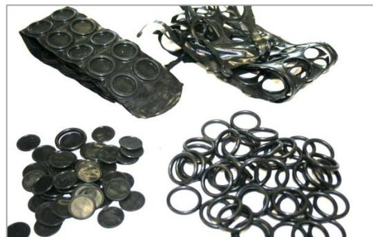
*Detail showing deflashed parts – first item is before deflashing and the SpinTrim separates into three parts including finished item (shown bottom right)*
