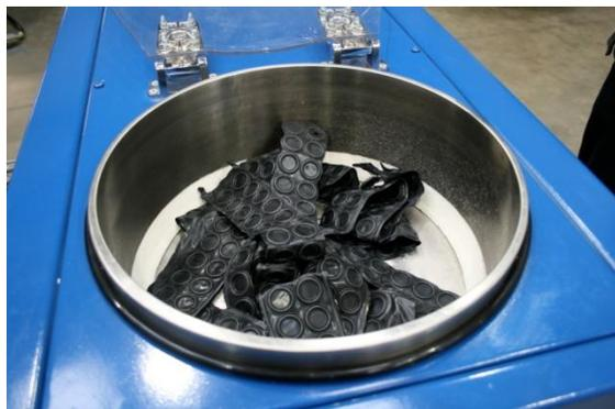
*Parts about to be released and dropped into spinning chamber*
